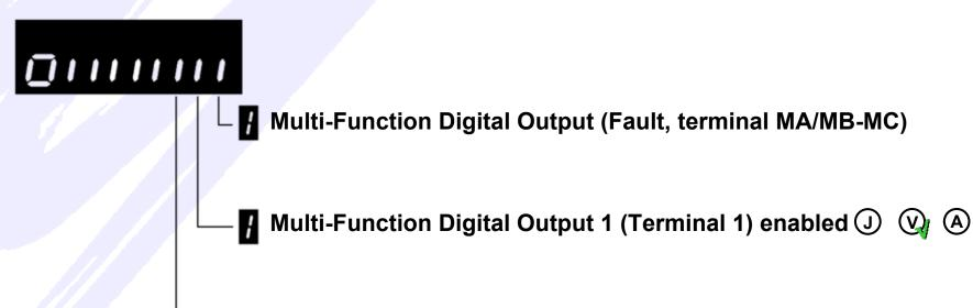
Multi-Function Digital Output 2 (Terminal 2) enabled
